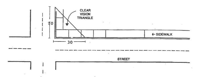
2. Vision Triangle at Driveway and Street Intersections: Where a driveway or alley enters the street right-of-way a vision triangle shall be formed by measuring 20 ft. into the lot as measured from the sidewalk edge that is closest to the property line (or from the property line if no sidewalk exists), and thirty feet (30') along the sidewalk edge (or property line if no sidewalk exists) parallel to the street.
